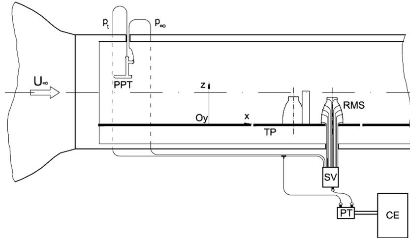
**Figure 5 Experimental setup utilized for wind loads measurements on the SDT rigid models 1:150 placed in the BLWT-AWEL: PPT – Pitot-Prandtl tube; RMS – rigid model at reduced scale; SV - scanning valve; PT – pressure transducer; CE – computing equipment:  $p_t$  - total pressure;  $p_\infty$  – static pressure**
