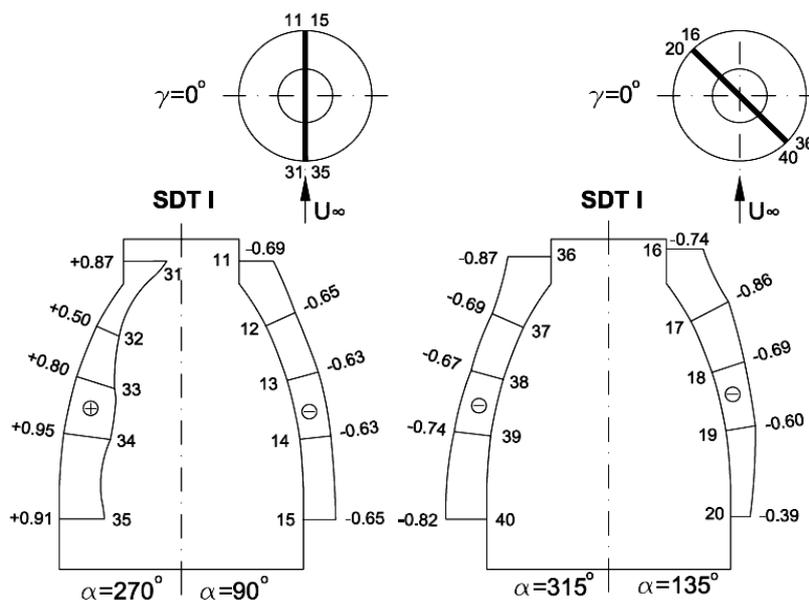
**Figure 7 Vertical cross section plots of the local pressure coefficients  $C_p$  distributions for the active SDT I of the model ensemble 1:150 scale**
