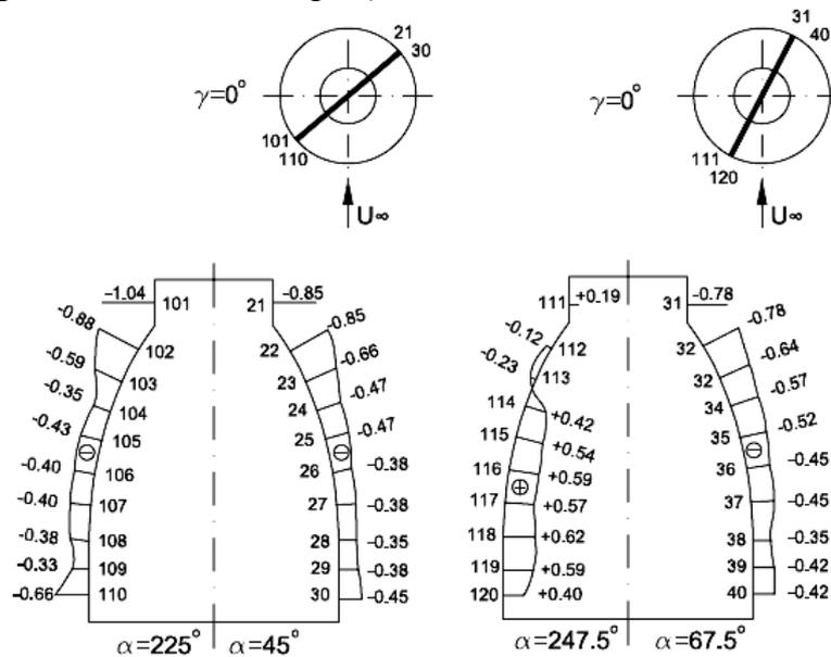
**Figure 6 Vertical cross section plots of the local pressure coefficients  $C_p$  distributions for the single SDT 1:100 scale model**
