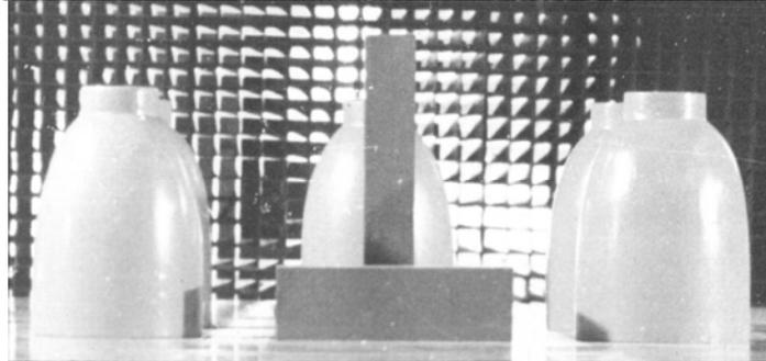
Figure 3 SDT ensemble - the five tanks, the process building and the access tower (1:150 scale)
