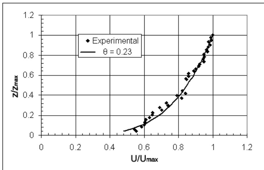
**Figure 1 Mean velocity profile in the experimental zone of the BLWT**
