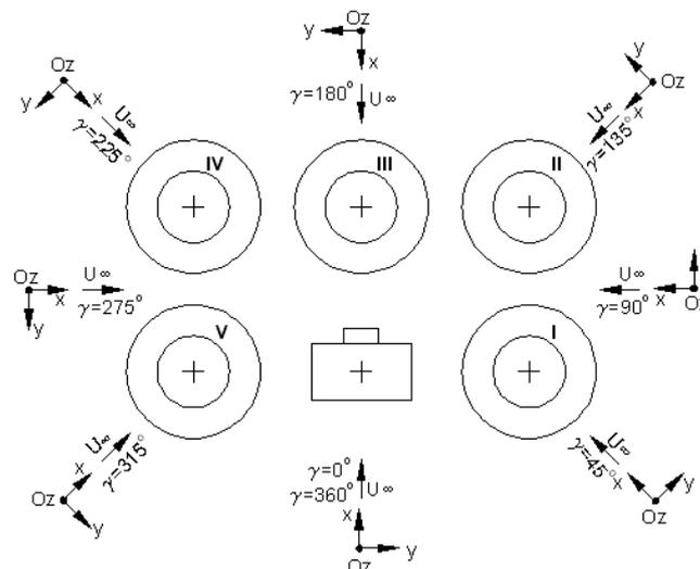
Figure 4 Modeled ensemble scheme specifying the position of each SDT, the other buildings and the wind-SDT incidence angles  $\gamma$
