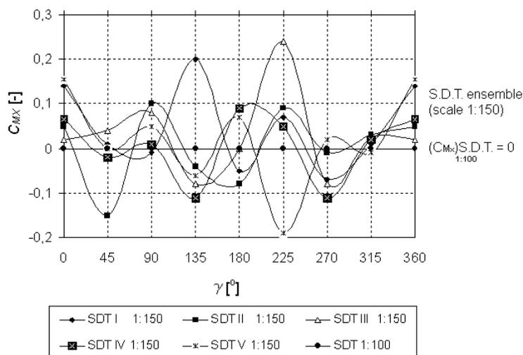
Figure 9 Variation graph of the aerodynamic momentum coefficient  $C_{M_x}$  with respect to the incidence angle  $\gamma$  and the SDT position in the ensemble
