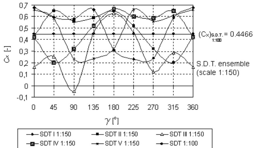
Figure 8 Graphical representation of the aerodynamic drag  $C_x$ , coefficient variation with respect to the incidence angle  $\gamma$  and the SDT position in the ensemble
