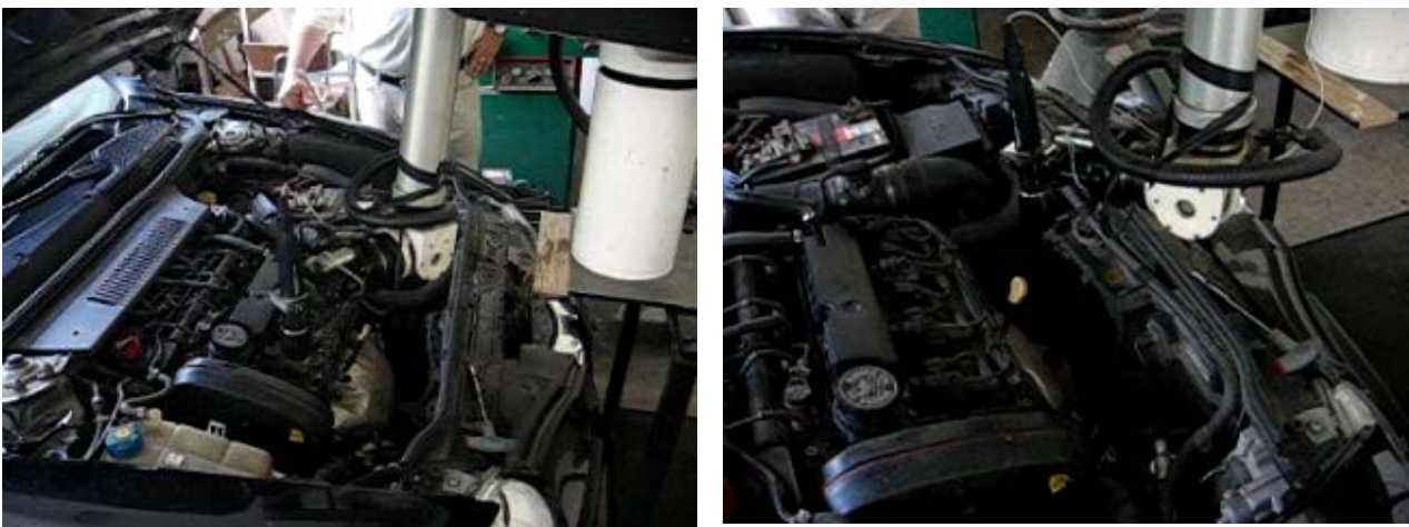
Fig.2. Pictures of robot arm with microphone in two different positions above the IC engine .
