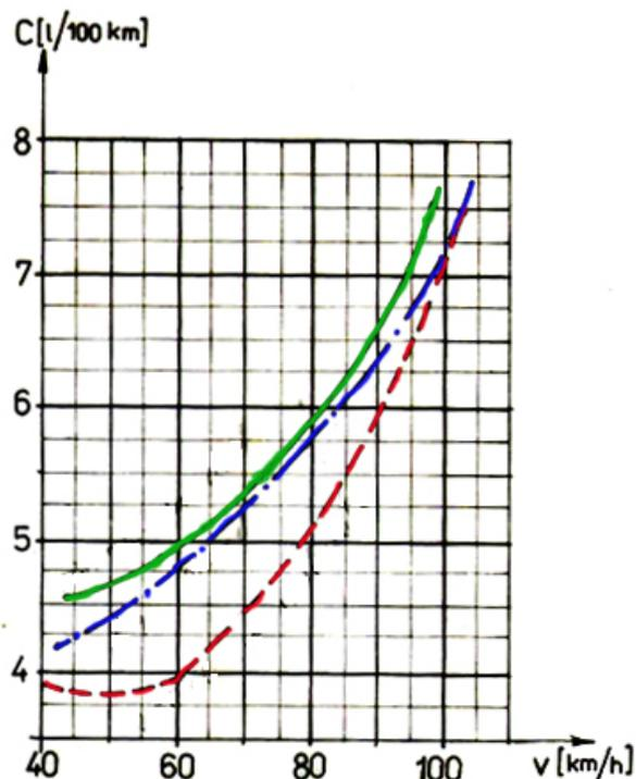
Fig. 7. Comparative consumption diagrams on the roll stand
