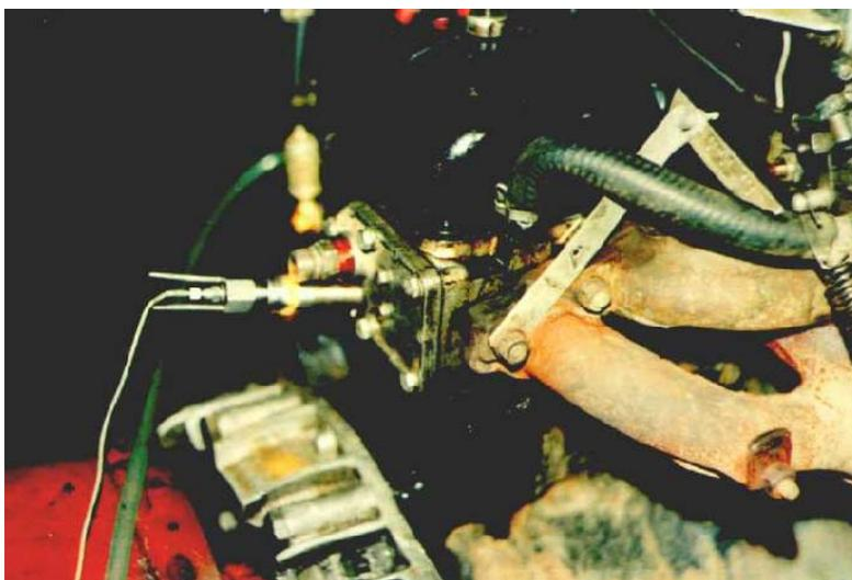
Fig. 3. Kistler 601 piezoelectric transducer for measuring the pressure in the cylinder
