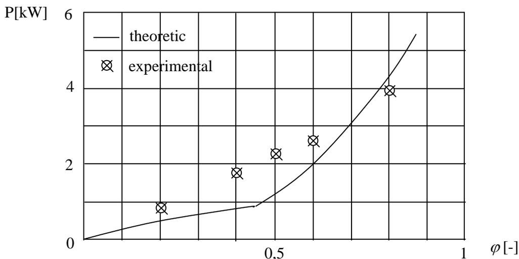
Figure 2 The dependence between mill net power of the vibrating mill and its filling coefficient
