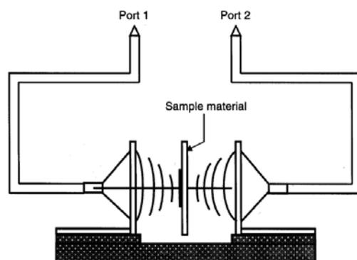
**Fig. 3. Schematic of a free-space transmission technique for measuring reflection and transmission (Ports 1 and 2 are connected to the Vector Network Analyzer).**
