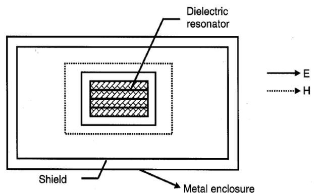
**Fig. 2. Schematic of an open cavity (TE013) dielectric resonator**
