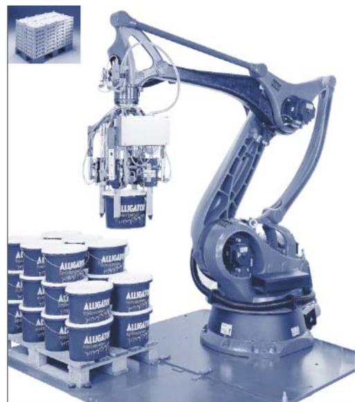
**Figure 2: Work cell for pail palletizing**
