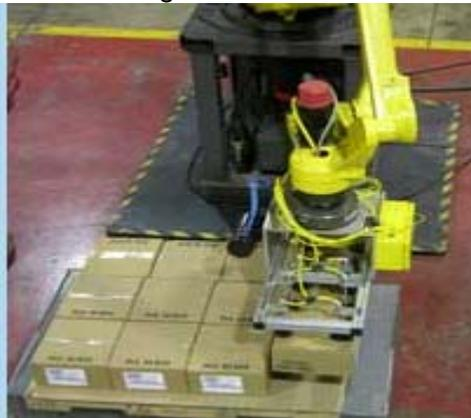
**Figure 7: Real environment box palletizing**
