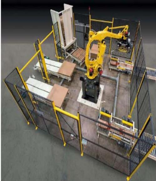
**Figure 1: Work cell for bag palletizing**
