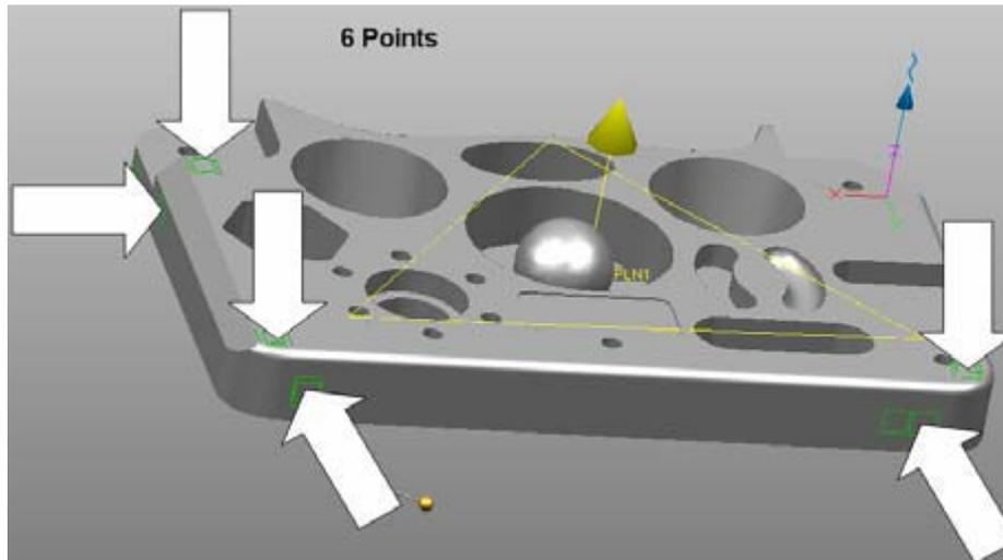
Fig.1 . The alignment six points surface
