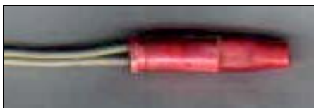
Figure 6. Drain plug injected on rheophores.
