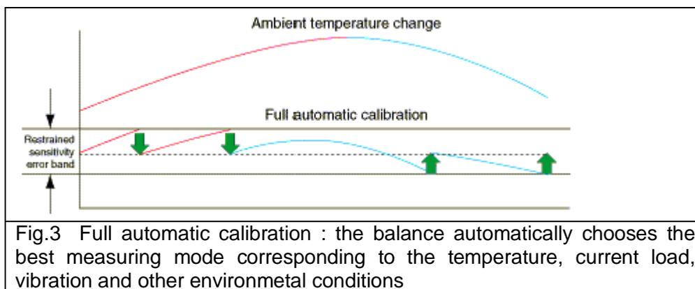
Fig.3 Full automatic calibration : the balance automatically chooses the best measuring mode corresponding to the temperature, current load, vibration and other environmental conditions
