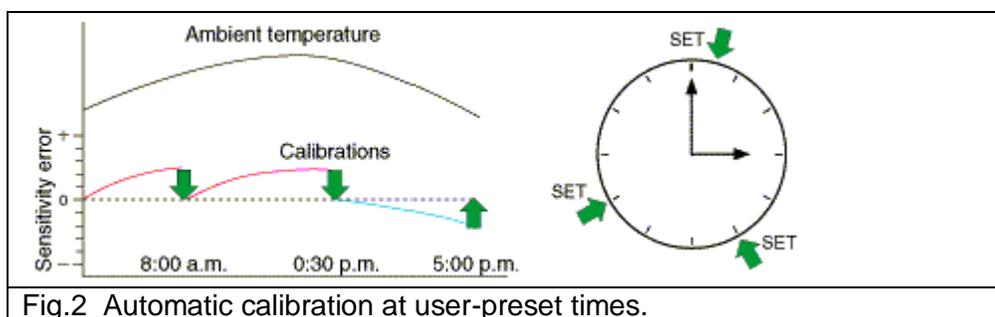
Fig.2 Automatic calibration at user-preset times.
