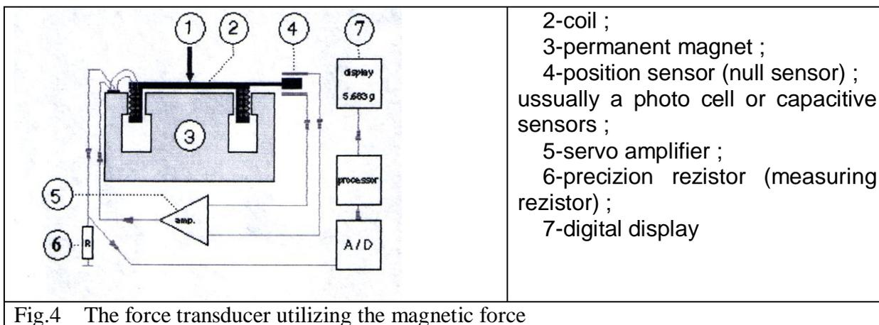
The force on the weighing pan is compensated by the permanent magnet and the magnetic field generated by the current in the coil. This current is regulated by the sensitive position sensor and the servo amplifier, and measured over the precision resistor by the analog-digital converter. The balance measures the current needed to keep the pan in its position and the pan does not move. [2]
