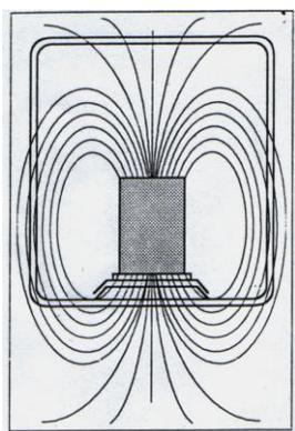
The magnetism of a weighing sample can lead to the weighing result being dependent on the position of the weighing sample on the weighing pan and to a result that is difficult to reproduce.
