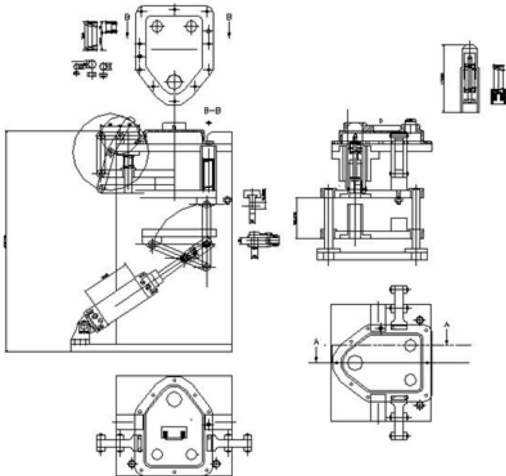
*Figure .5. Fixing scheme of the semi product in the orientation and fixing device.*
