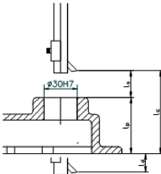
Figure .2. The determination of the work-piece  $l_c$  length scheme.
