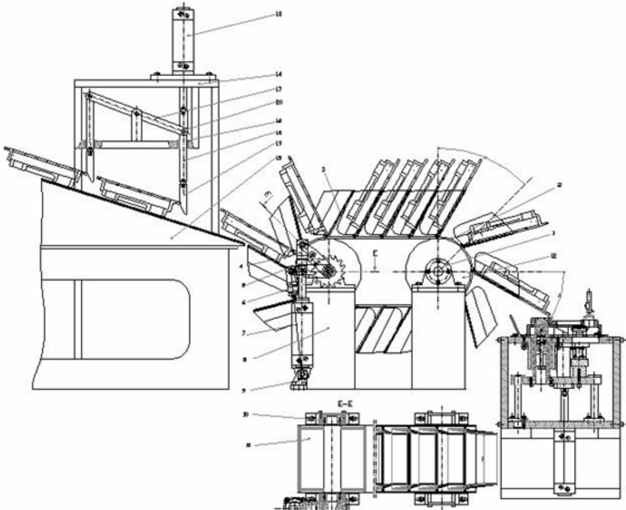
*Figure.6. the 2D assembly drawing of the transfer device integrated in a flexible processing system.*
