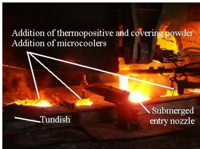
*Figure 2 Places for addition thermoisolating and covering powders and of microcoolers in tundish*
