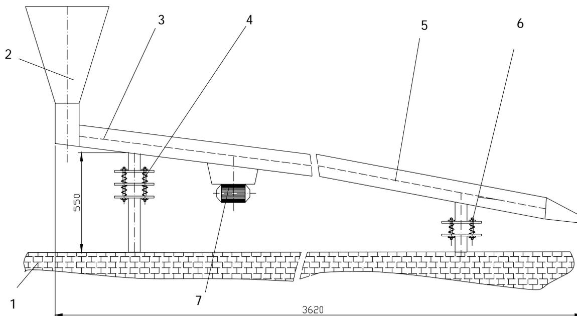
**Figure 5 Experimental installation for addition of microcoolers in the tundish and crystallizer of the continuous cast installation**
