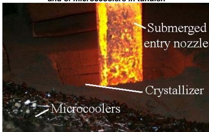
*Figure 3 Places for addition of microcoolers in crystallizer*
