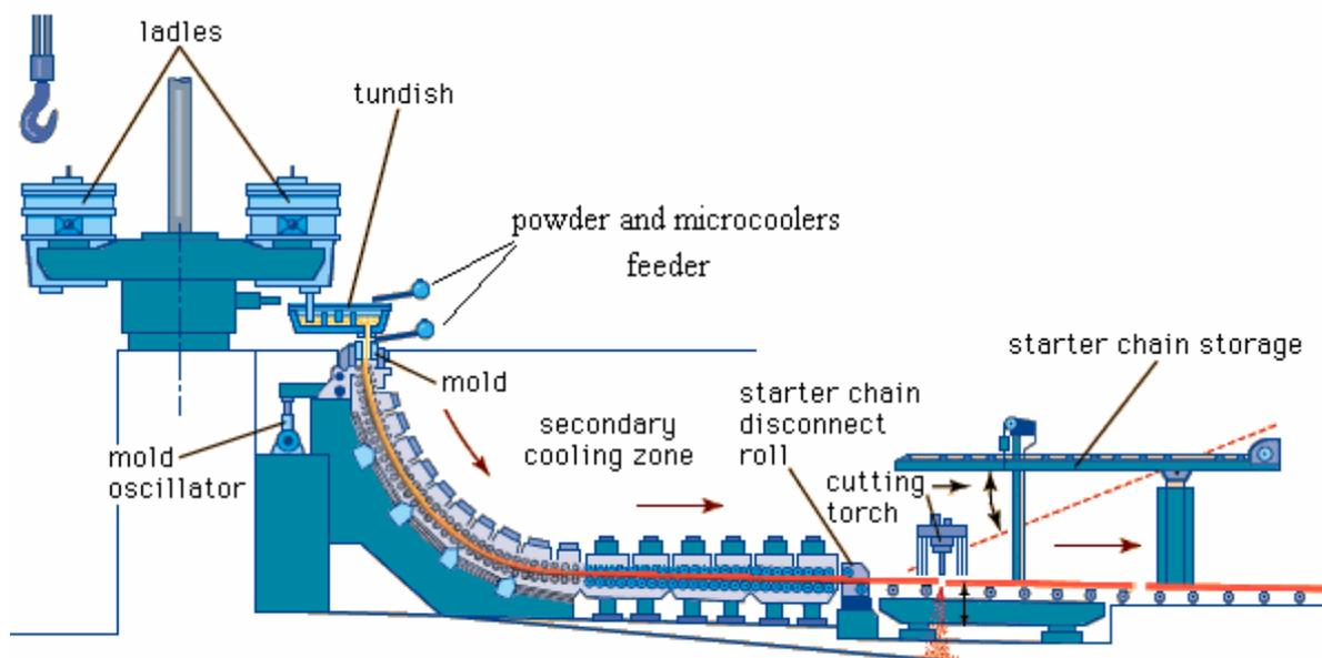
*Figure 1 Continuous casting installation*
