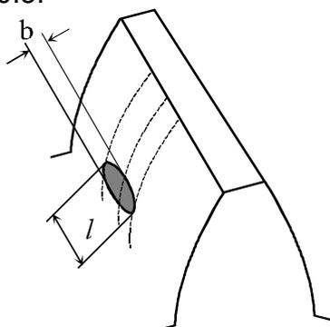
**Figure 2. The shape of the flattening ellipse**
