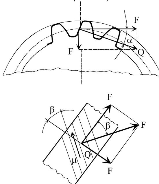
**Figure 1. The forces in the grinder-gear gearing**
