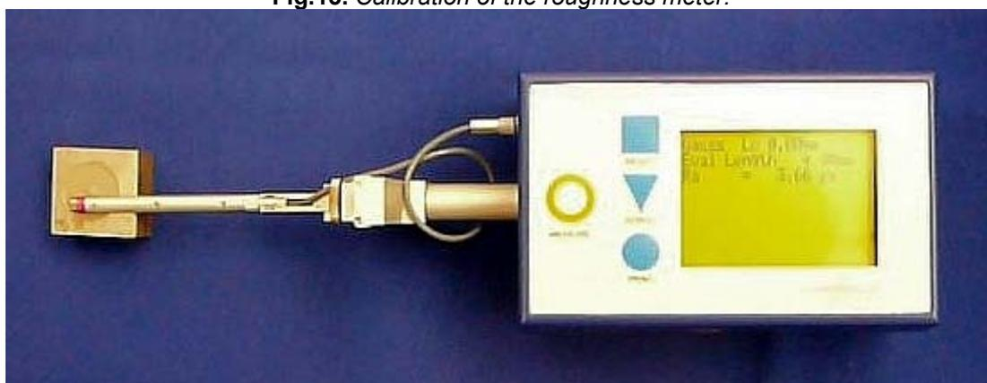
Fig.16. Measuring of an electrical discharge worked piece.
