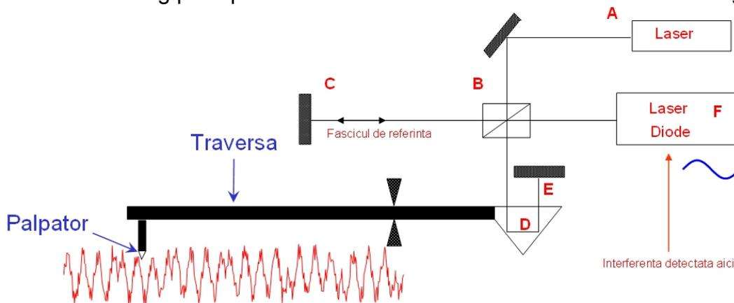
Fig.10. Laser interferometer sensing head.
