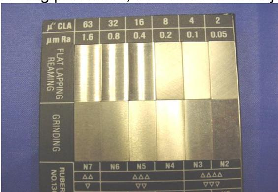
Fig.4. Roughness gauge for chipping worked surfaces.
