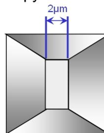
Fig.12. Truncated pyramid shaped pin.
