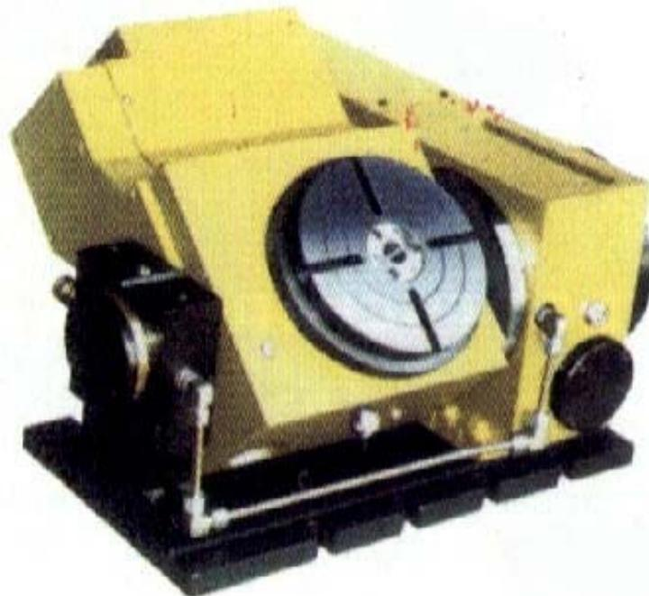
Fig. 5 – The rotary-tilting table with 2 CNC axes, as detachable unit
