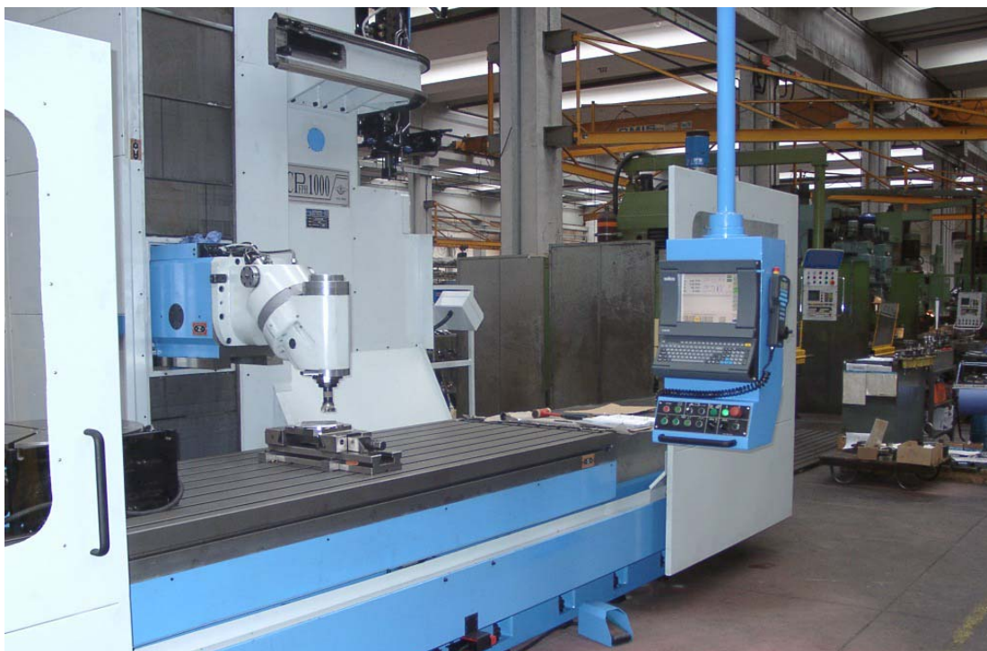
Fig. 1 – CPFPH 1000 with H/V automatic milling head and CNC positioning rotary table, [1].
