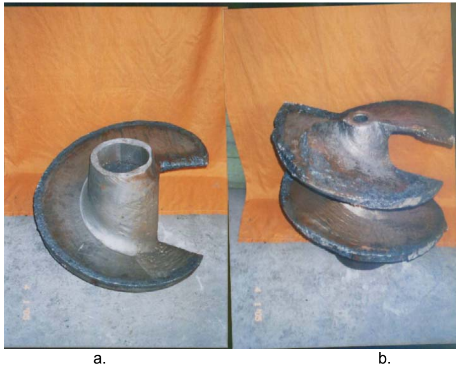
Fig. 6 The spiral, after having been surfaced with the buffer-layer: a – only one helix; b – with two helixes
