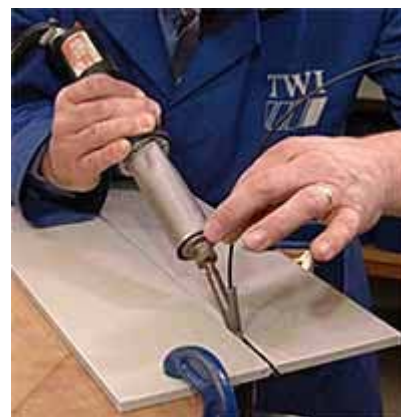
Fig.1. Hot gas welding
