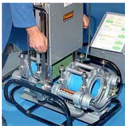
Fig.3. Butt fusion welding
