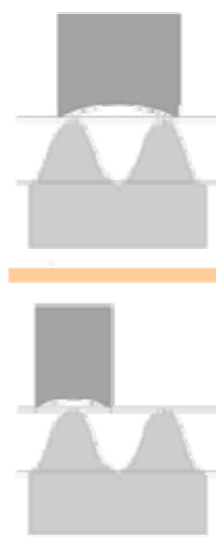
Figure 1. While superfinishing can put a mirror finish on the part, it may also be used to improve roundness, depending on the incoming roundness of the workpieces and the width of the stones. Narrow stones (at left, above) ride up and down on the lobes to improve surface finish only. Wider stones (at left, below) can bridge the lobes to reduce their depth (that is, to improve roundness) and impart a high degree of surface finish at the same time.
