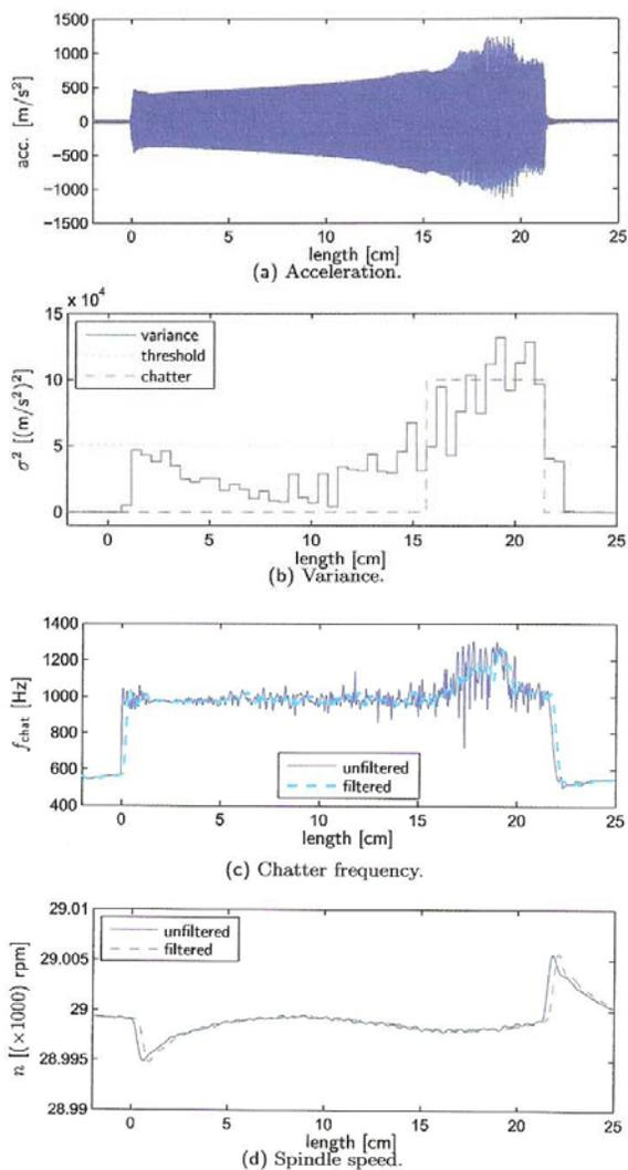
Fig. 5 The experimental results at 29000rpm, with  $a_p$  that increases from 4.0 to 6.0 mm. [36], [76]
