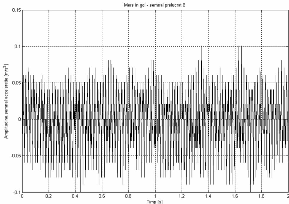
Fig. 9 Acceleration signal for beech wood processing at a revolution  $n=15000$ rpm
