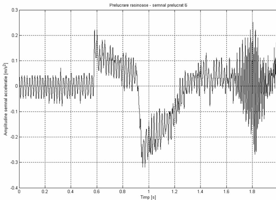
Fig. 8 Acceleration signal for resinous wood processing at a revolution  $n=15000\text{rpm}$  [76]
