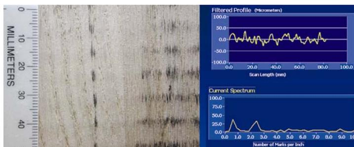
Fig. 2 The “imprint” of the regenerative vibrations on the processed surface in case of vibrations occurrence
