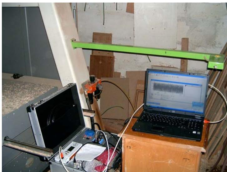
Fig. 3 The stand of measuring and control of the vibrations. Mounting and displaying the apparatus. (SC MOBIL SA Tileagd)
