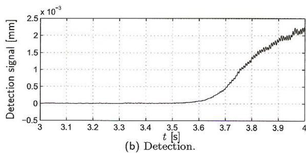
Fig. 4 Simulating the detection of vibrations at increasing the cutting depth
