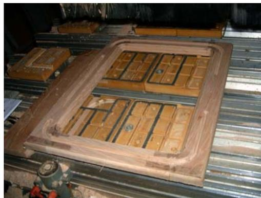
Fig. 1 The oak timber piece after processing. It can be noticed an absence of the effects of the regenerative vibrations (SC MOBIL SA Tileagd)
