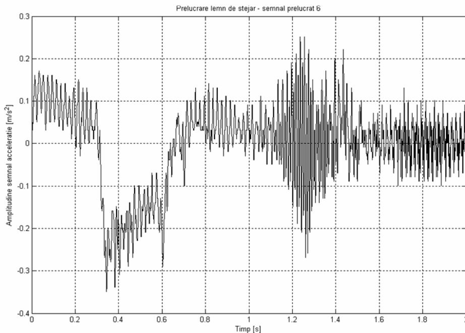
Fig. 7 Acceleration signal for oak wood processing at a revolution  $n=15000\text{rpm}$
