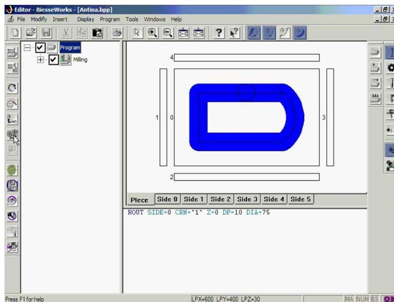
Fig. 13 Programming the processing parameters by cutting with the BiesseWorks program.[3]
