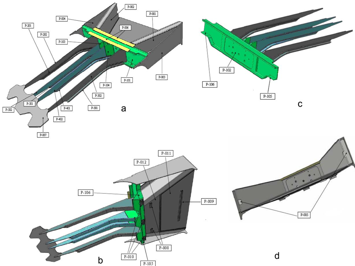
**Fig. 5. The location of the parts in the headboard assembly**
