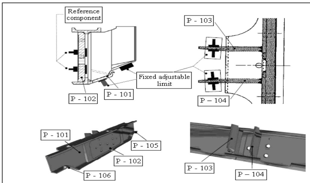
**Fig. 6. Positioning technological scheme for welding operations**
