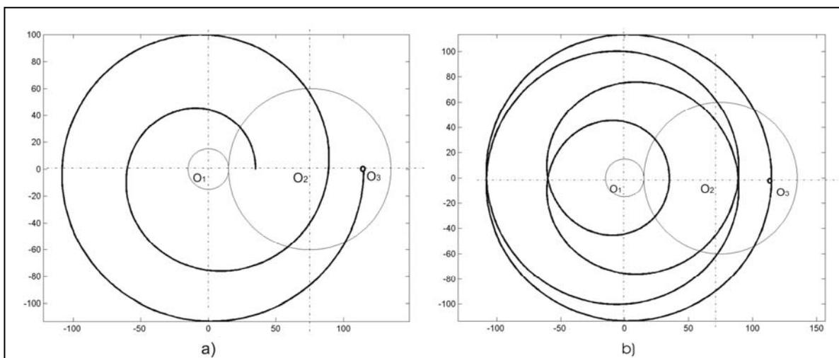
**Fig.4 Trajectories of metallographic probes in the rotation plane : a) 2 rolls on the fixed circle; b) 4 rolls on the fixed circle.**
