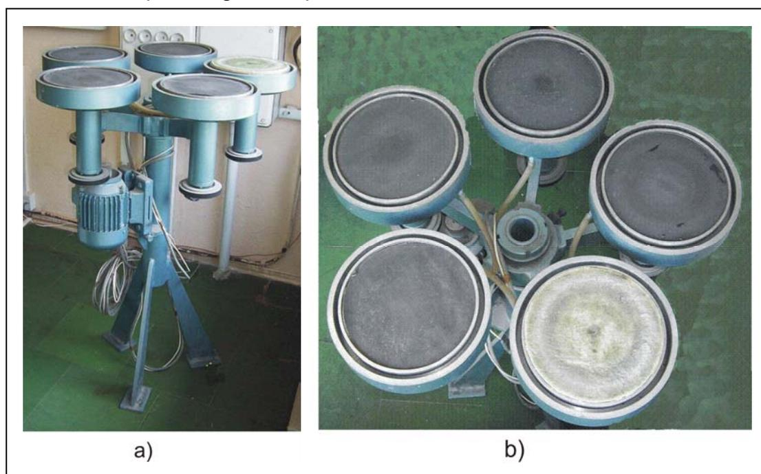
**Fig. 2 Metallographic probe finishing machine**
