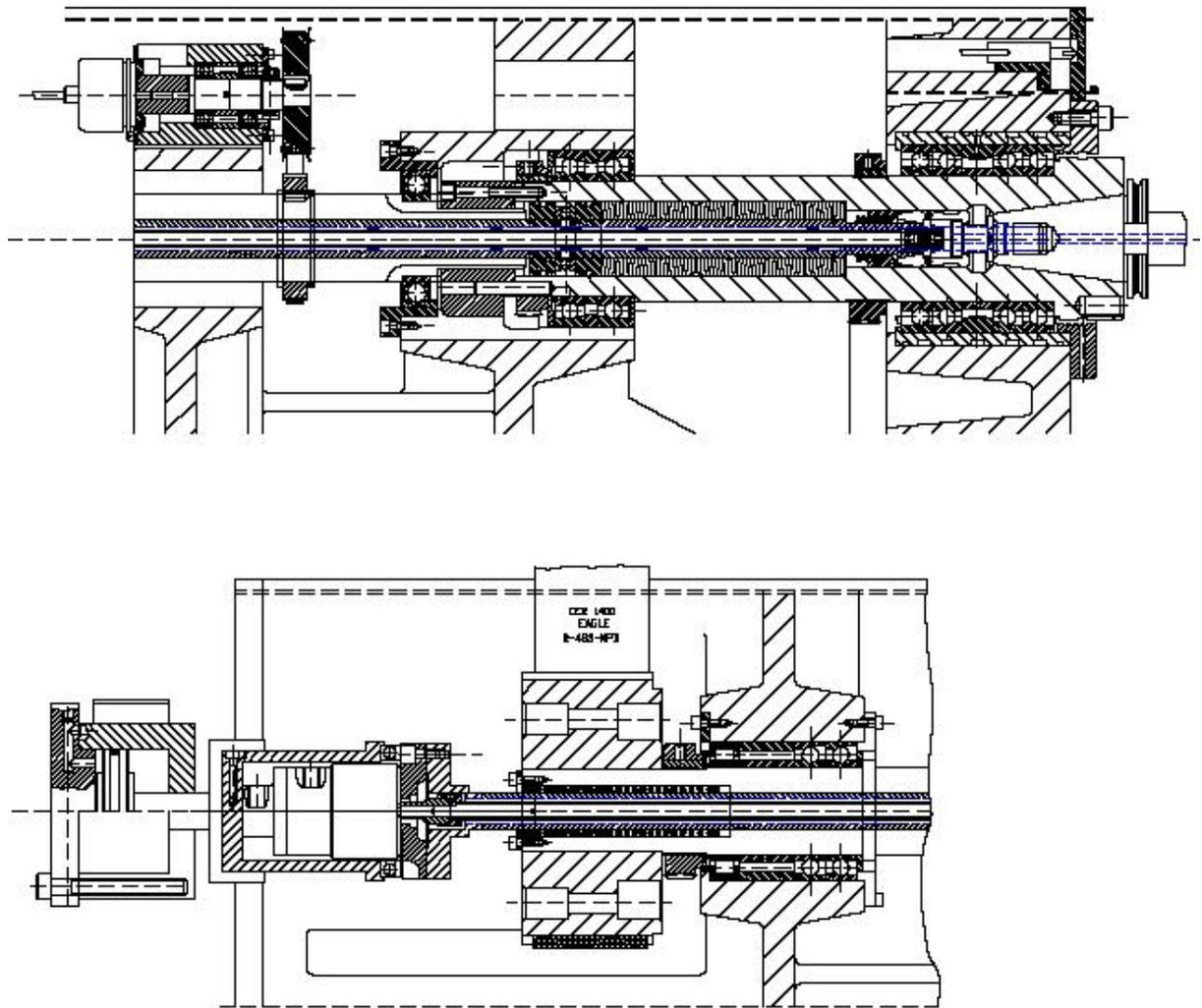
**Fig. 4 – The new main spindle inside of the ram**
