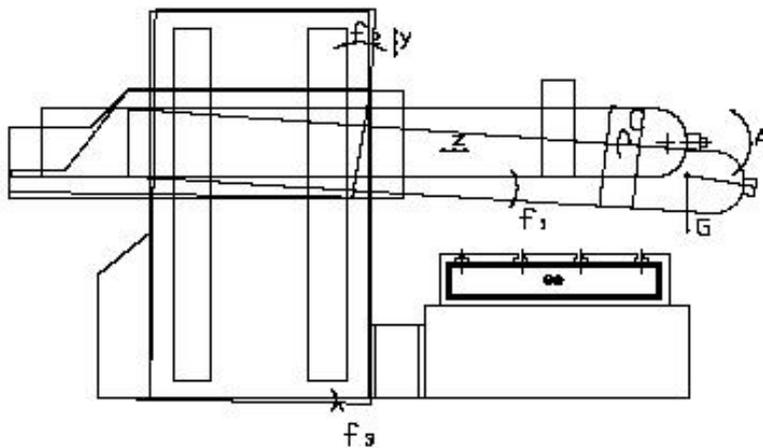
*Fig. 2 – The principle of the machine deformation under the ram weight*
