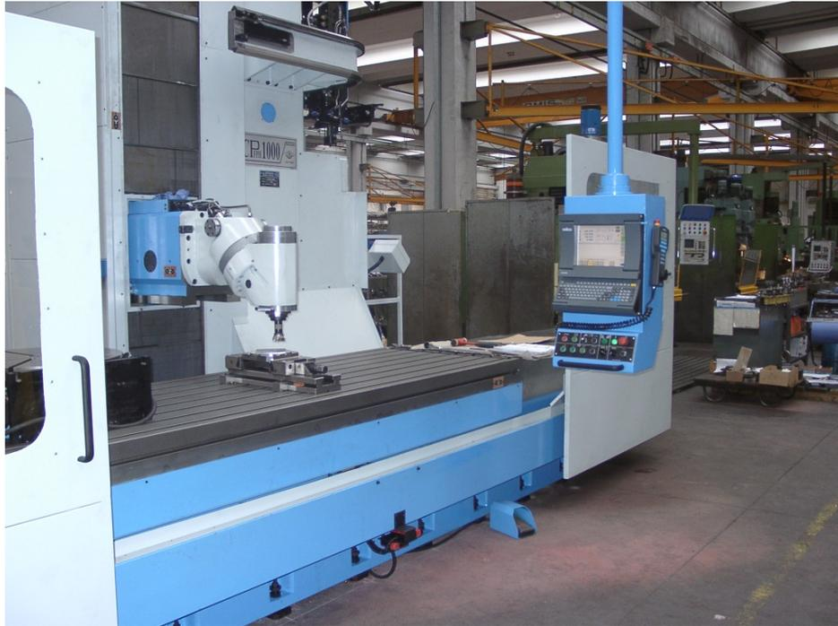
*Fig. 1 – CPFPH 1000, with H/V milling head, Stimin Oradea*
