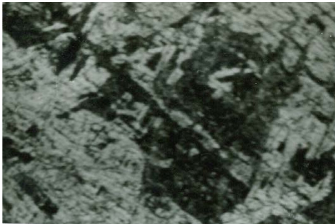
Figure 4. Microstructure, Nital 2%, x100 0% micro-coolers (the median area).
