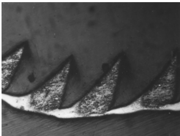
Micrography X150; Cutting test parameters: CM insert; a_1=0,1\text{mm} ; V_c=120\text{m/min} ; \gamma=-6^\circ ; no coolant
