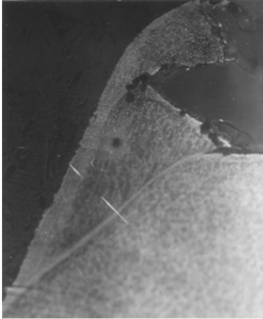
Micrography X250; Cutting test parameters: CM insert; a_1=0,1\text{mm} ; V_c=120\text{m/min} ; \gamma=-28^\circ ; no coolant
