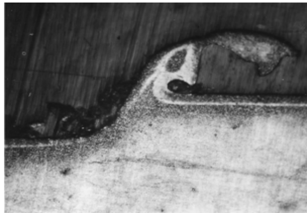
Micrography X200; Cutting test parameters: CM insert; a_1=0,1\text{mm} ; V_c=120\text{m/min} ; \gamma=-6^\circ ; VB=0,2\text{mm} ; no coolant
