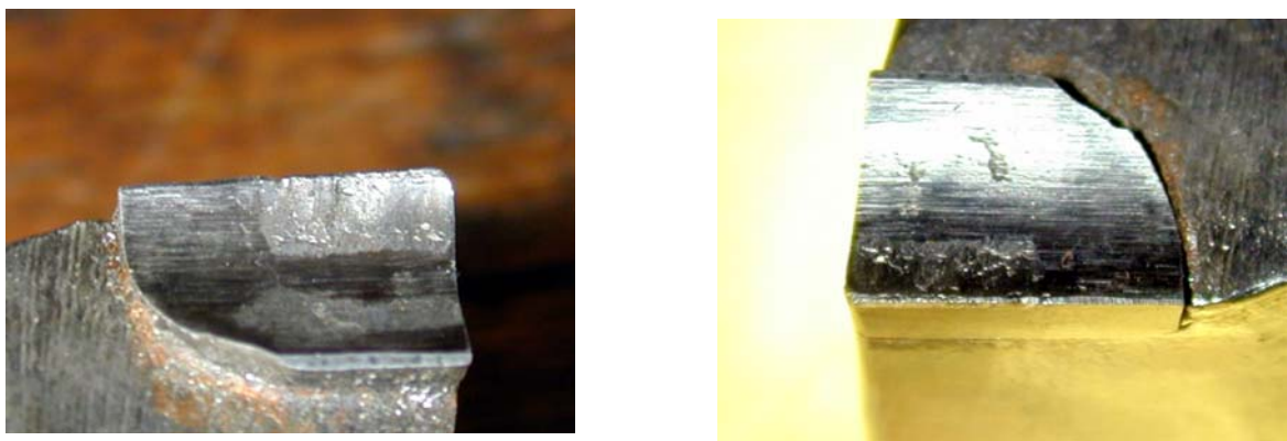
Figure 5: Diffusion wear of the cutting tool
