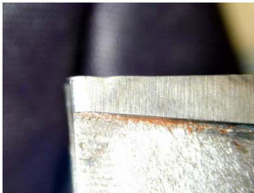
Figure 4: Abrasive wear of the cutting tool
