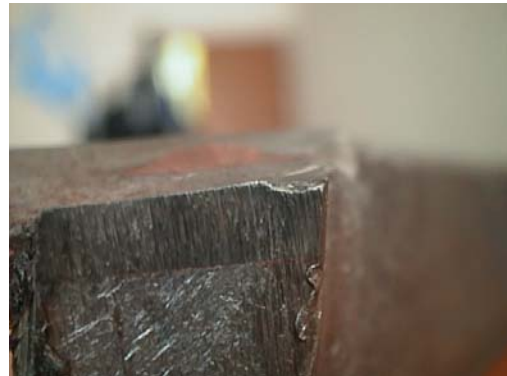
Figure 4: Abrasive wear of the cutting tool
