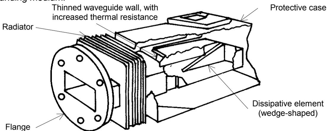
Fig.2. Dry calorimeter, for microwave power measurement.
