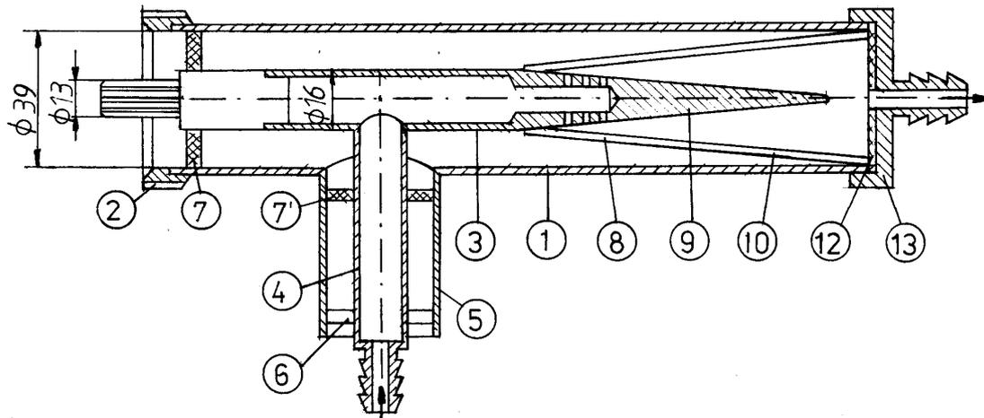
Fig.4. Water artificial load, used for microwave power up to 10 kW in the 2.45 GHz range.
