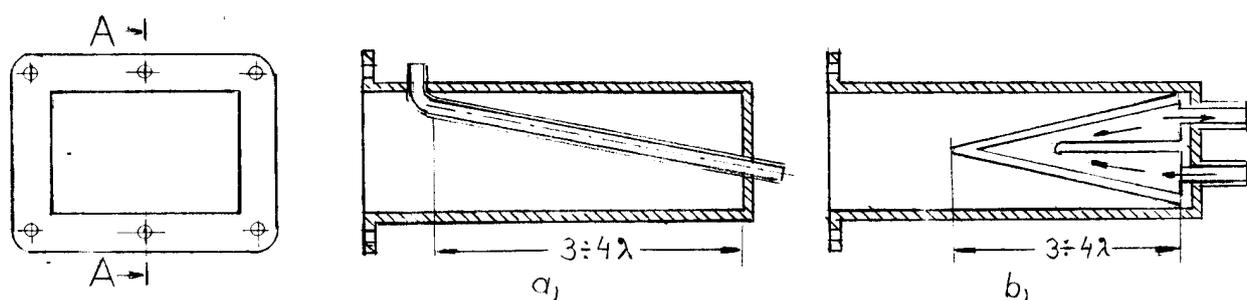
Fig.5. Terminal artificial loads, adaptable to the 109x54 mm rectangular waveguide.
