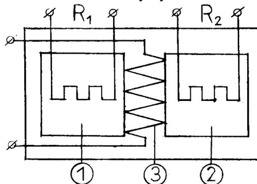
Fig.1. Principle of the double calorimeter user for microwave power measurement.
