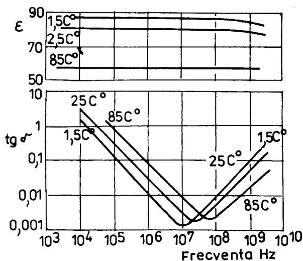
Fig.3. Variations of the water dielectric properties with frequency and temperature.
