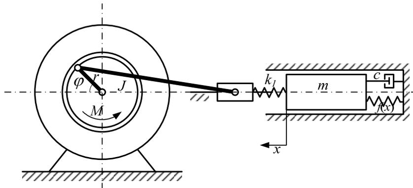
Fig.1. Dynamic model of mechanism
