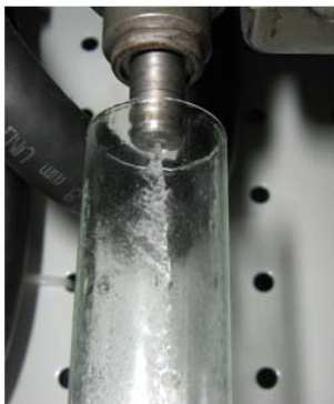
Figure 2: Picturing the fuel spray.
