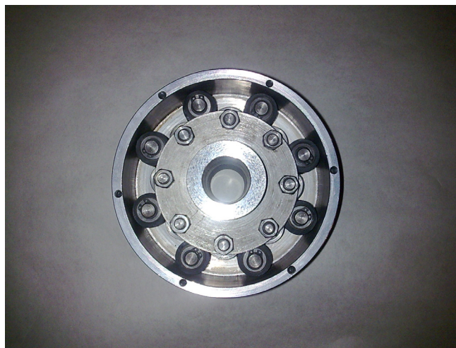
Fig.2 Elastic and safety clutch with metallic roles and elastic rubber elements.
