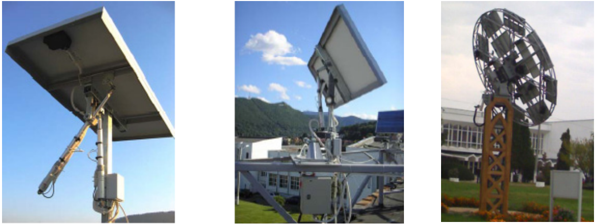
Figure 4. Tracking systems designed and implemented at Transilvania University of Braşov: a) pseudo-equatorial [3], b) azimuthal [15], c) pseudo-equatorial platform [5] b)
