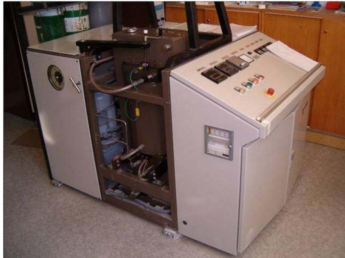
*Fig. 5 Hot Isostatic Pressing (HIP)*
