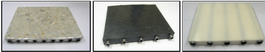
Figure 7. Prototypes manufactured with COMPUTER ABS, PP1B and PVC respectively
