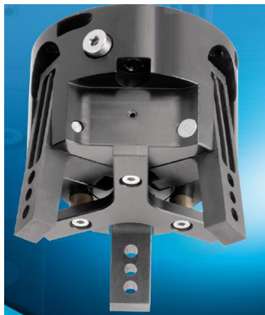
Fig.5. Present the tree finger angular gripper for the arm of the robot [14]
