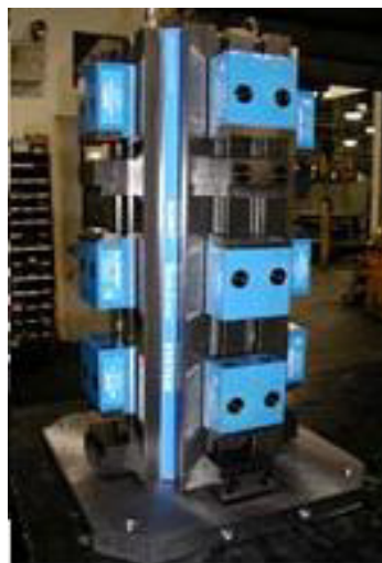
Fig.4. Modular fixture system with 2 device level [14]
