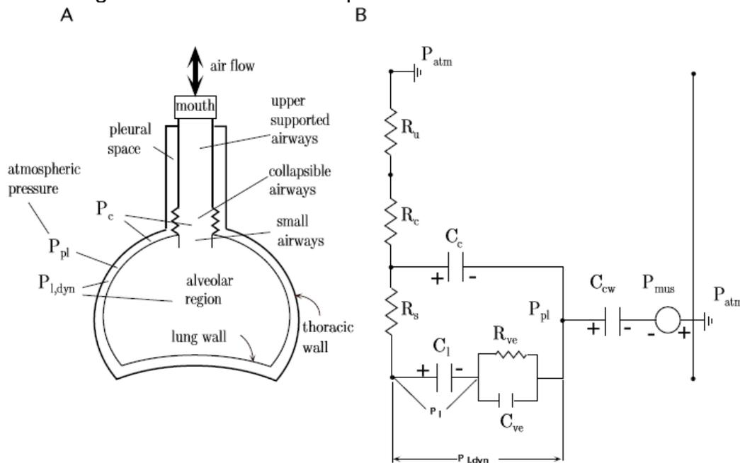
**Fig.5. Physical model of respiratory system (A) and pneumatic analog model (B) proposed by Athanasiaides et al, [6]**
