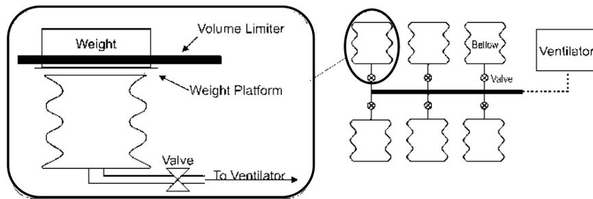
**Fig.2. Mechanical model of the lung, Chase et al., [3]**
