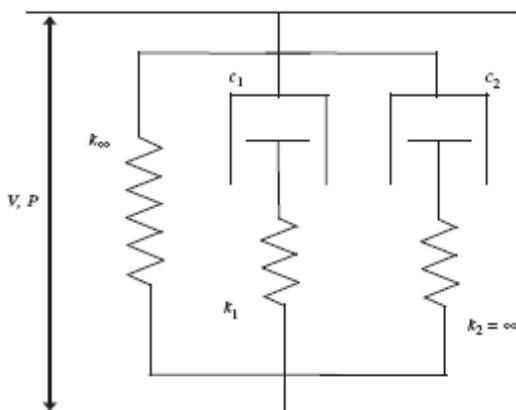
**Fig.7a. Mechanical viscoelastic model, [8]**
