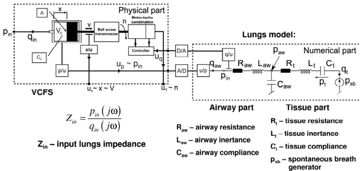
**Fig.4. The hybrid lung model of Kozarski et al. [ ]**
