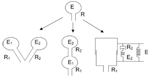
**Fig.9. The single-compartment linear model and its three two compartment extensions: parallel model (left), series model (middle) and viscoelastic model (right), Bates and Lutchnen, [11]**
