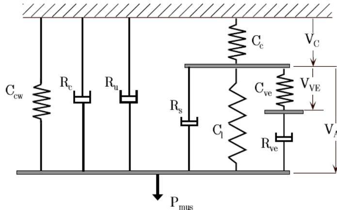
**Fig.6. Mechanical equivalent of respiratory mechanics model, Athanasiades et al, [6 ]**
