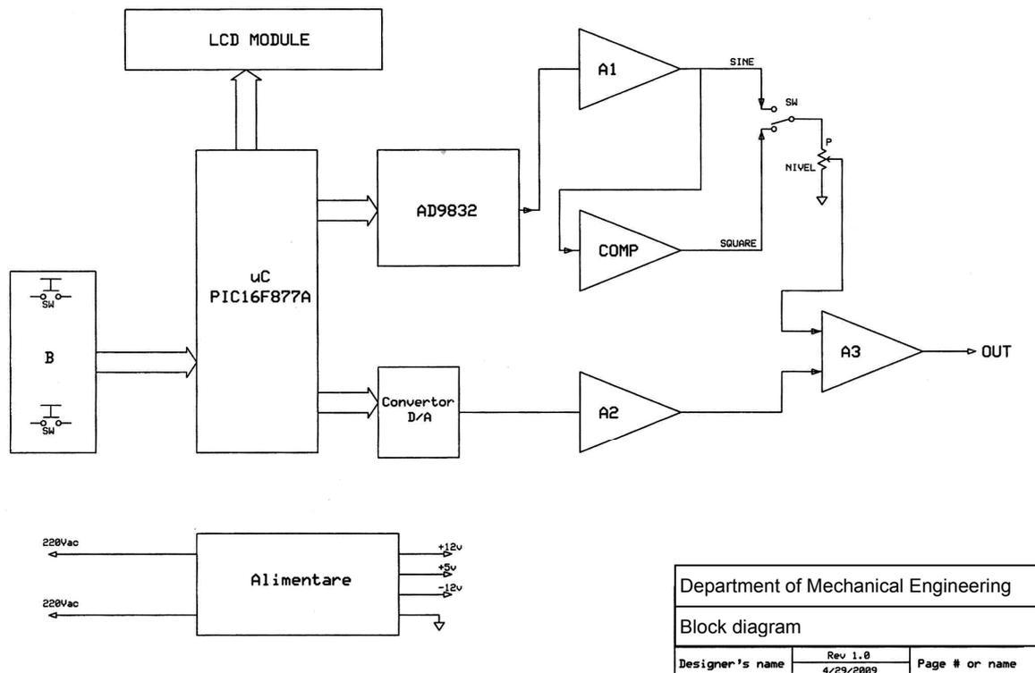
**Figure 1: Block diagram of function generator with PIC 16F877A**
