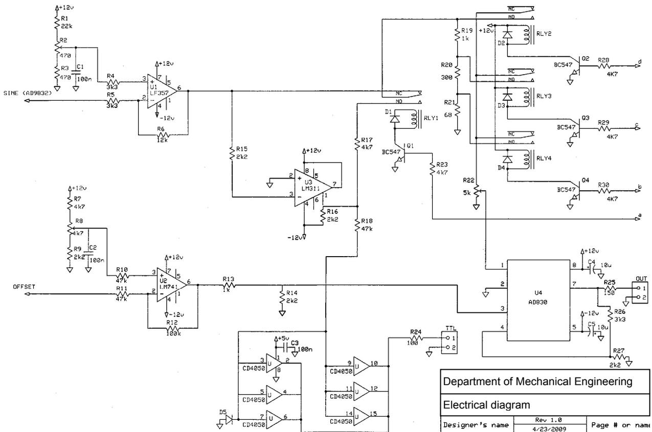
**Figure 2: Electrical diagram of the functions generator.**
