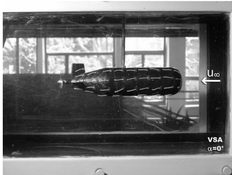
Fig. 5 The flow visualization in the boundary layer through the “method of wires”
