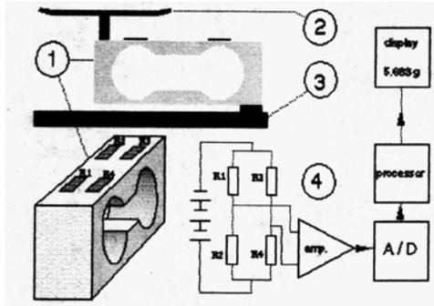
**Fig.1 Operational schemes of electronic balances with strain gauges**
