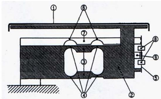
**Fig.2 Electronic Balance Sensor type vibrating string**
