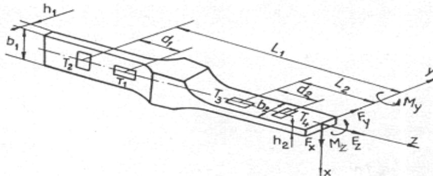
**Fig.4 Sensitive element for the displacement determination on two direction**
