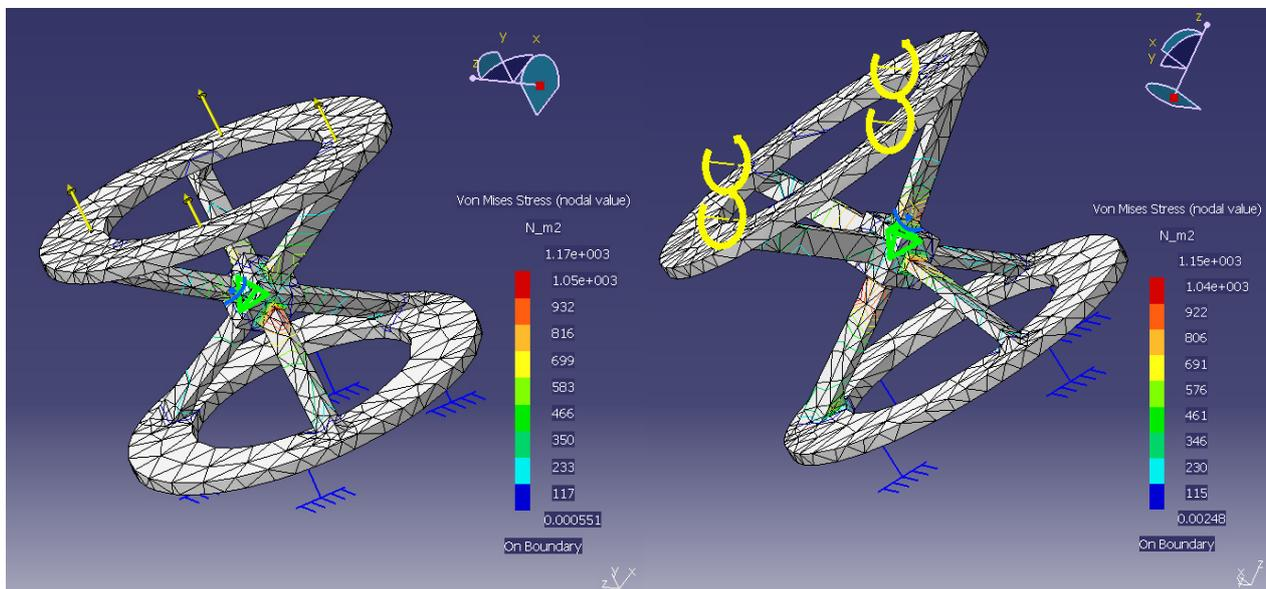
**Fig. 5 The tensions and deformation of the Y axis ( $F_y$ ,  $M_y$ )**
