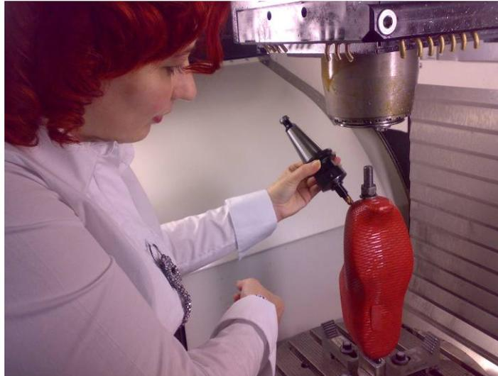
**Figure 12 - Positioning of the last and finger-type cutter for processing**
