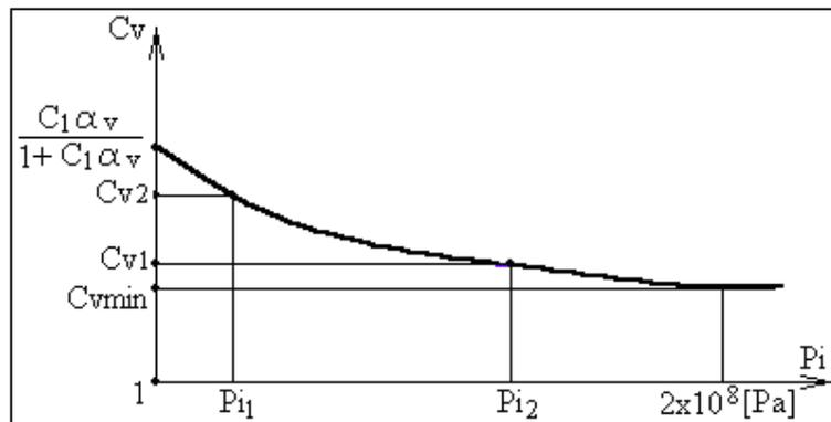
**Fig.3. The graphic of shrinkage variation with holding pressure.**
