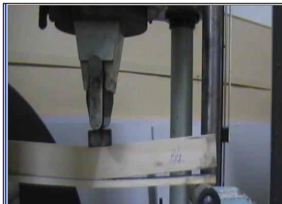
**Fig.3 Tension failure of a reinforced wood beam with one CFRP plate and a slide of wood**
