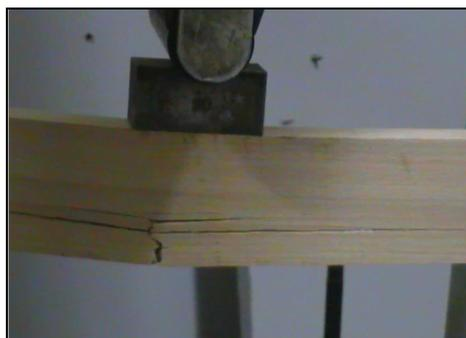
**Fig.1 Tension failure of an un-reinforced wood beam**
