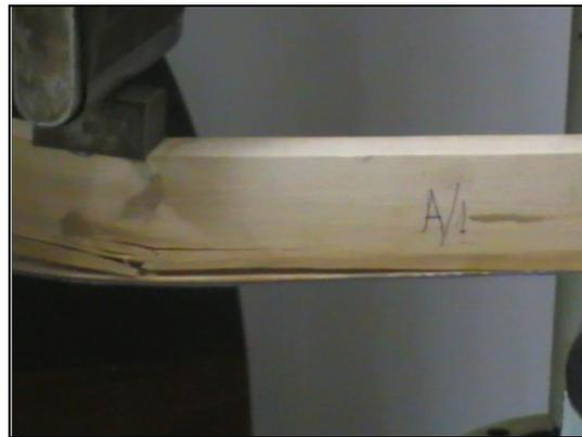
**Fig.2 Tension failure of a reinforced wood beam with one CFRP plate**
