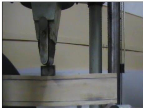
*Fig.4 Tension failure of a reinforced wood beam with two CFRP plates and two slides of wood*
