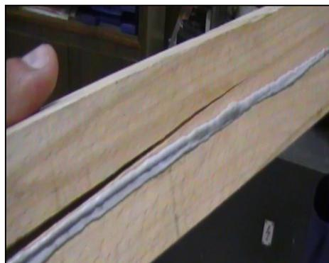
*Fig.5 Tension failure of a wood beam reinforced with epoxy resin*
