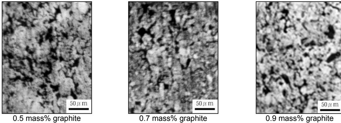
**Figure 5. Microstructures of steam treated specimens**
