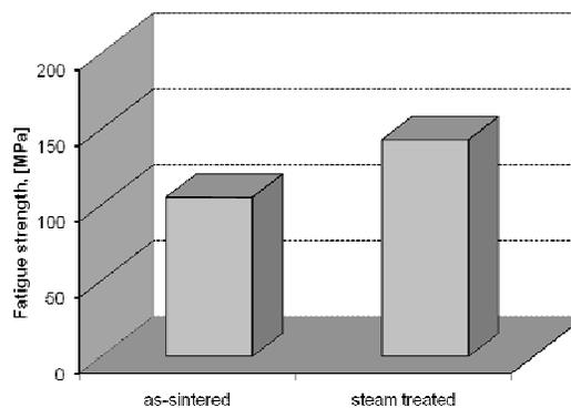
**Figure 2. Comparison of fatigue strength**
