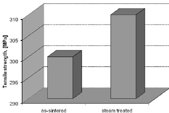
**Figure 1. Comparison of tensile strength**
