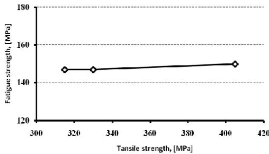
**Figure 6. Relationship between tensile strength and fatigue strength of steam treated specimen**
