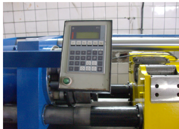
Fig. 4. MSF-40 Machine: a – expander – blade detail; b – panel for the command and adjustment of the welding parameters
