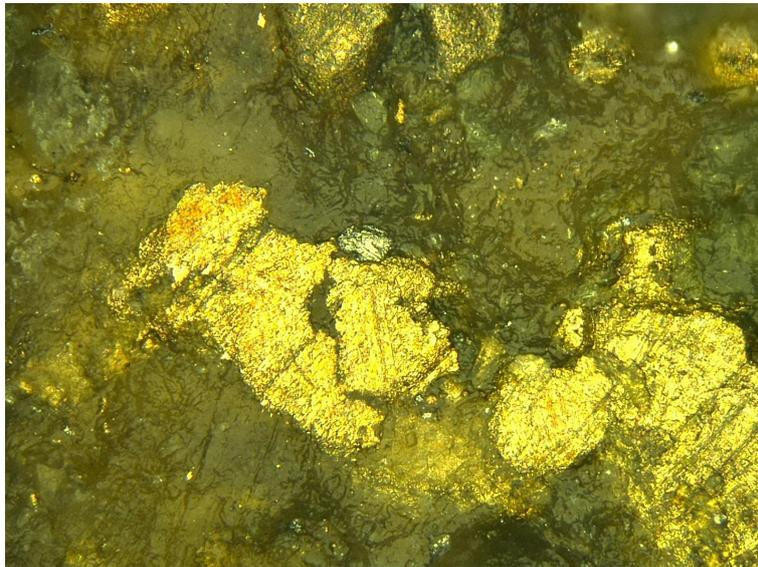
**Fig. 1 Micrographic view of a 60% copper reinforced polymeric composite sample (x500 magnification)**
