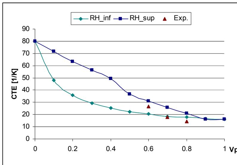
**Fig. 4 Theoretical predicted (Rosen-Hashin models) and experimentally retrieved CTE values for all the copper reinforced polymeric composites**
