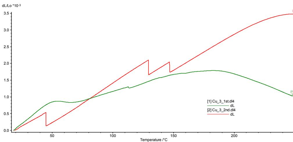
**Fig. 5 Thermal strain variation with temperature for two successive heating cycles applied upon the 80% copper reinforced composite sample**
