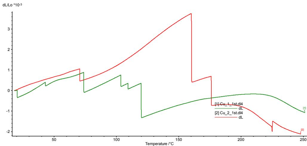
**Fig. 2 Thermal strain variation with temperature for 60% and 70% Cu reinforced polymeric composites – first heating cycle**
