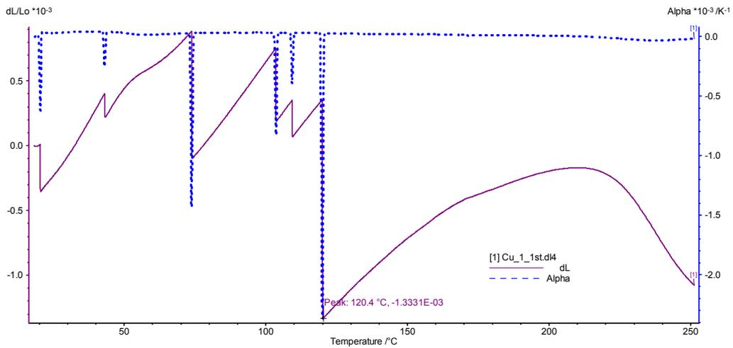
**Fig. 3 Thermal strain and coefficient of thermal expansion variations with temperatures for the 60% Cu polymeric composites – one heating cycle**
