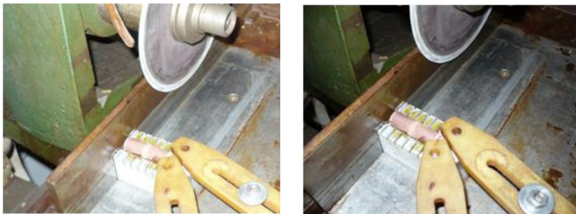
Fig.2 Device for cutting the sintered basalt pieces
