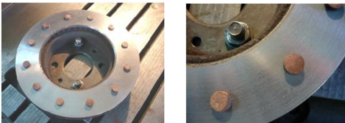
Fig.5 Attaching basalt sintered pellets into brake disk closed holes
