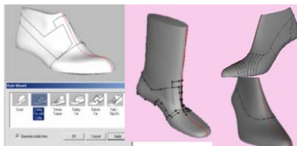
Fig. 5 Creating style-line on the last surface with this 'user friendly' using session of application Shoe Design
