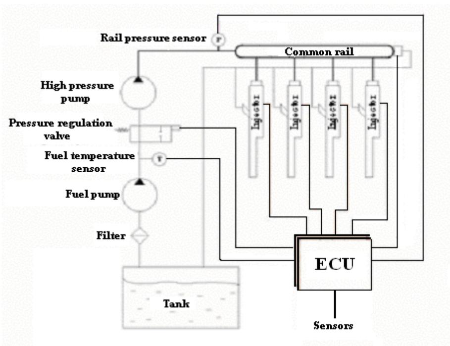
*Fig.1 Common rail injection system*
