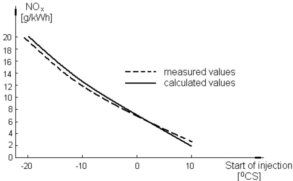
Fig.4 Comparison between measured and calculated values for nitrogen oxides
