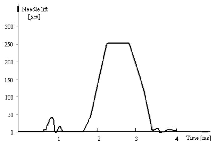
*Fig. 3 Needle lift*
