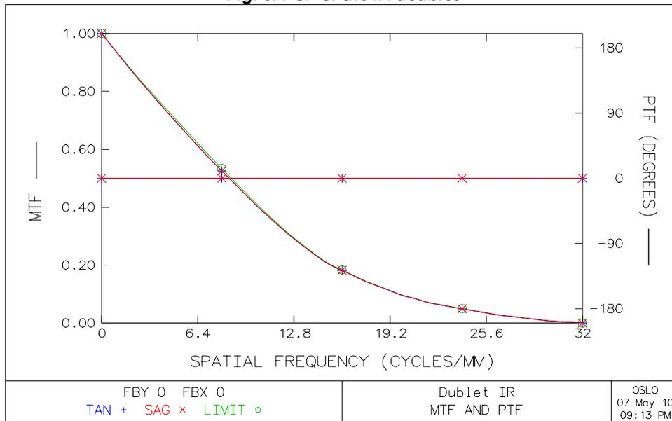
**Fig. 6. MTF and PTF of the IR doublet**
