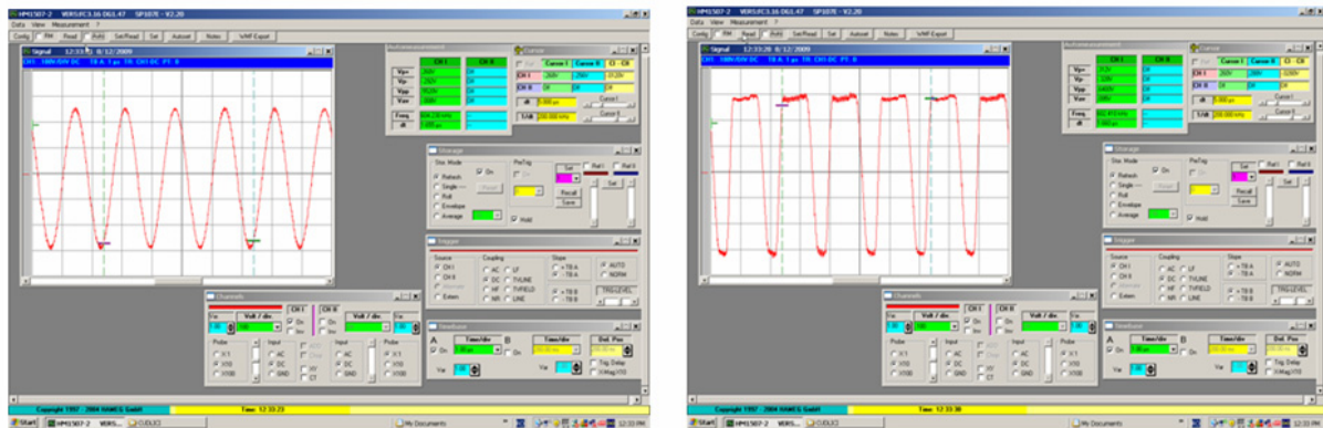
Fig. 5: Sine and square wave 300 kHz – 10 V at 2 V/div.
