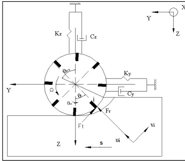
**Fig.4. Dynamic model of peripheral milling process [11,12]**
