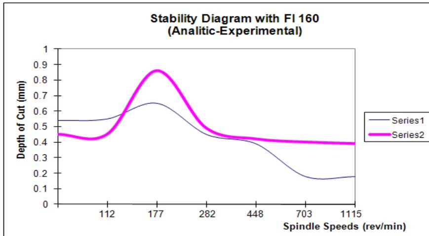
**Fig.5: Stability diagram of milling process by used cutter FI160 for  $K_t=983$  N/mm<sup>2</sup>; Series1-experimental mode, Series2-analytical mode**
